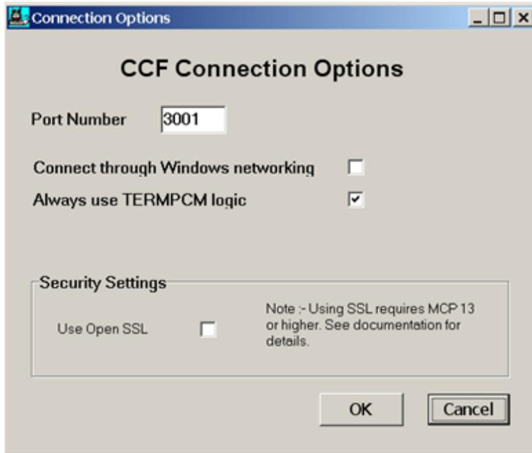
The **Port Number** tells C.A.T.T. which port to use when opening a connection. This must match the port number used on the MCP. If not, your connection attempt will fail with a “timeout” error.
