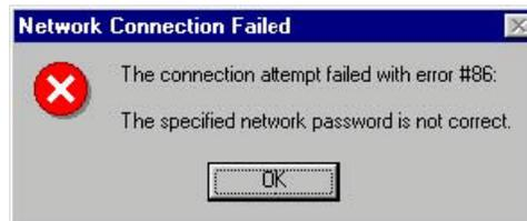
In this case, you must connect to the MCP host using *Windows* first.<sup>1</sup> After successfully opening a share to the MCP from *Windows*, and saving the password, then you can attempt to reconnect using C.A.T.T.
